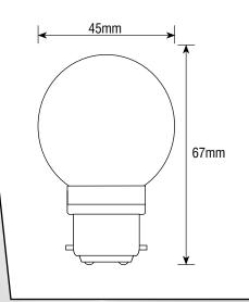
An LED direct replacement to the golf ball lamp, offering outstanding lamp life and efficiency. The range includes white, coloured and colour changing golf balls. Using no more than 1W of power these lamps have very low power consumption, and are highly efficient. They are ideal for festoon lighting, inaccessible areas and applications where long lamp life is essential.
