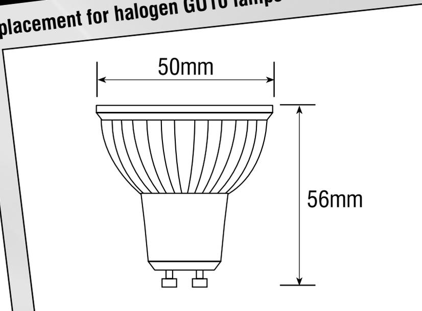
Prolite are now able to offer a high power LED cluster lamp. This lamp has an innovative design and is installed into a standard GU10 halogen body for 100% retro-fit installations. Available in a range of colours.
