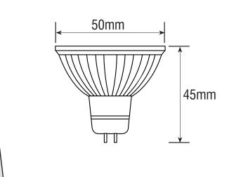
This LED cluster lamp has an innovative design and is installed into a standard MR16 halogen body for 100% retro-fit installations. Available in a range of colours. Requires a compatible LED driver.
